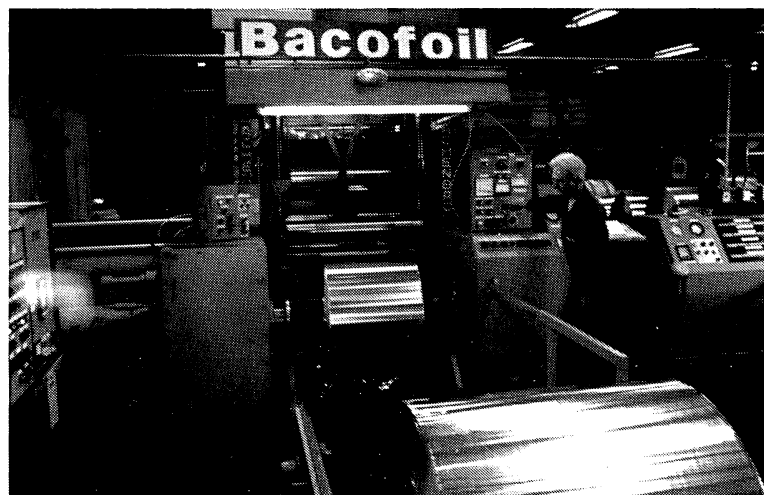
Figure 1 Passing coiled aluminium sheet through rollers to reduce it to the required thickness for foil.
