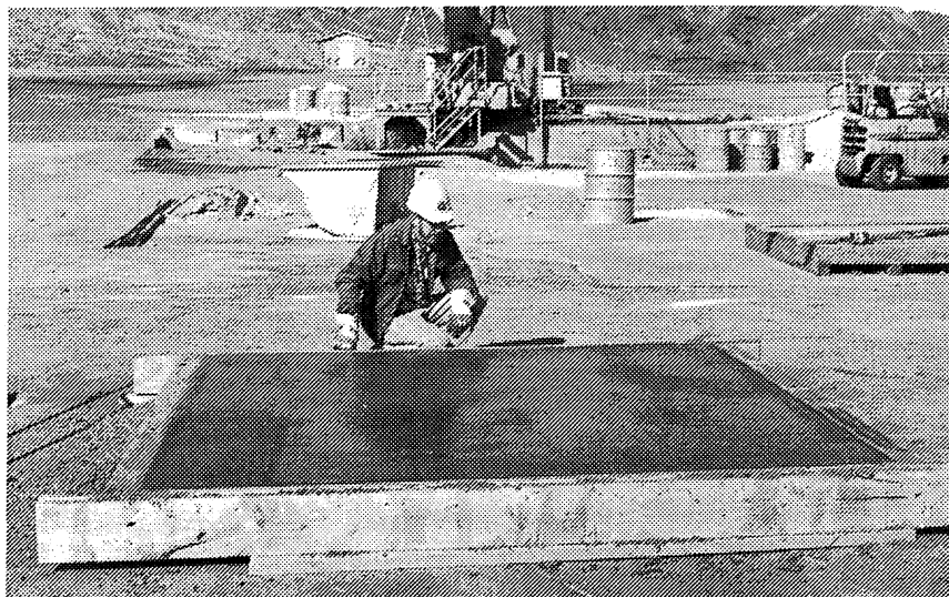
Figure 1 A slab of sulphur concrete
