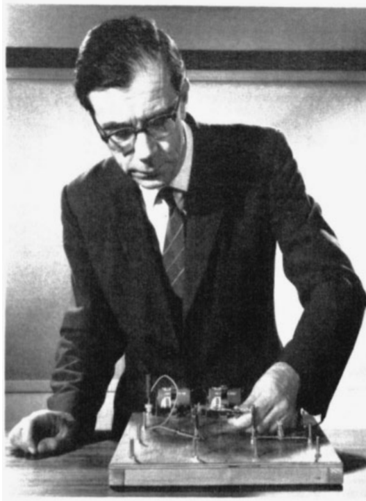
Figure 3 The Worcester circuit board is used by 12-year-old pupils to learn about elementary electrical circuits from first-hand experience. Here they are shown how they could 'blow' their fuse of wire wool. (From the Esso film The Worcester Circuit Board .)
