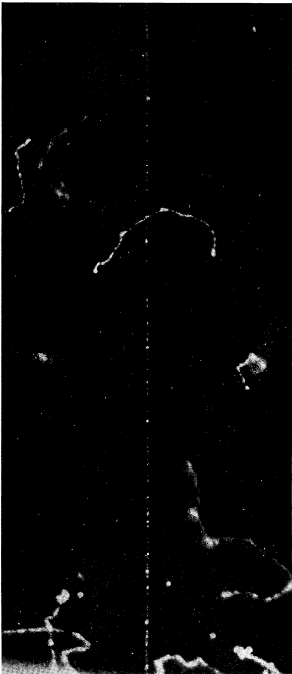
Beta particle tracks. One fast particle crossed the tracks of several slow ones. C. T. R. Wilson (1923) Proc. Roy. Soc., A, vol. 104, Pl. 16. Photo, Science Museum, London.
