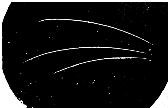
Alpha particle tracks in a very strong magnetic field. P. Kapitza (1924) Proc. Roy. Soc., A , vol. 106, Pl.9.
