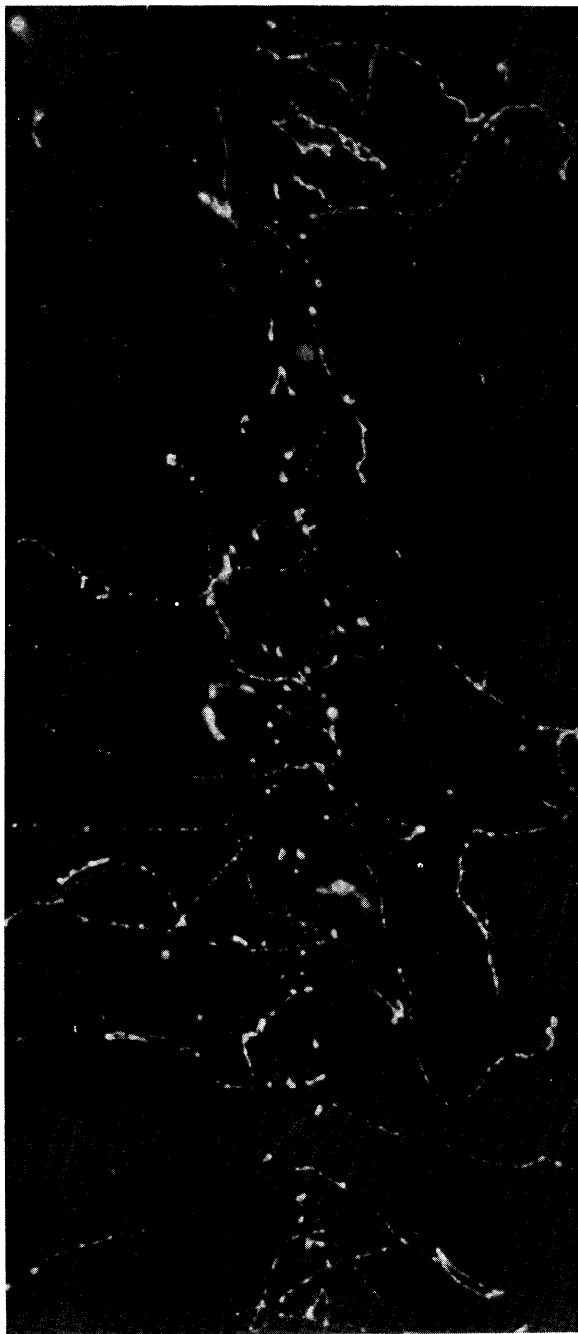
X-rays passing through wet air eject electrons which leave tracks. Gamma rays produce a similar effect with longer tracks. C. T. R. Wilson (1912) Proc. Roy. Soc., A, vol. 87, Pl. 8.
