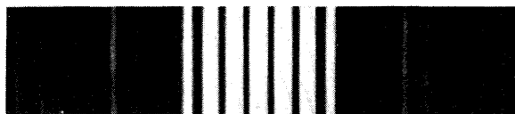
D A double slit interference pattern of light. R. S. Longhurst (1973) Geometrical and physical optics. Longman.
