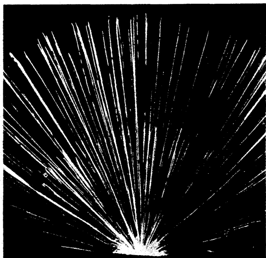
Alpha-rays from a small source: a mixture of thorium C and C'. Note there are two lots of alpha-rays, each with a definite range in air. (J. Chadwick.) From Radioactive Substances and Their Radiations , by Rutherford, Chadwick, and Ellis; Cambridge University Press.
