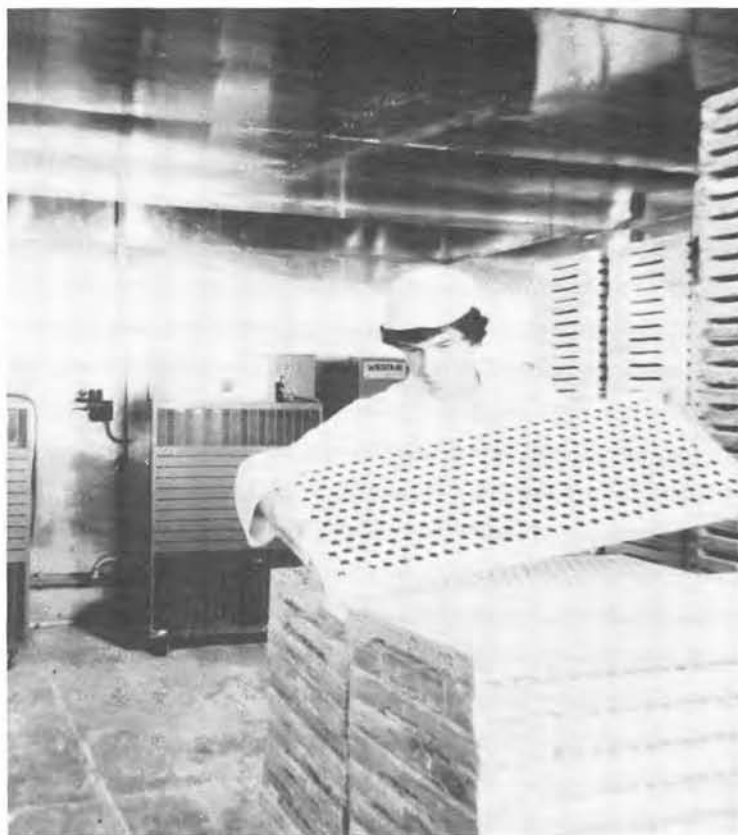
Figure 2 The heat pump dehumidification chamber at Smith Kendon. The Electricity Council
