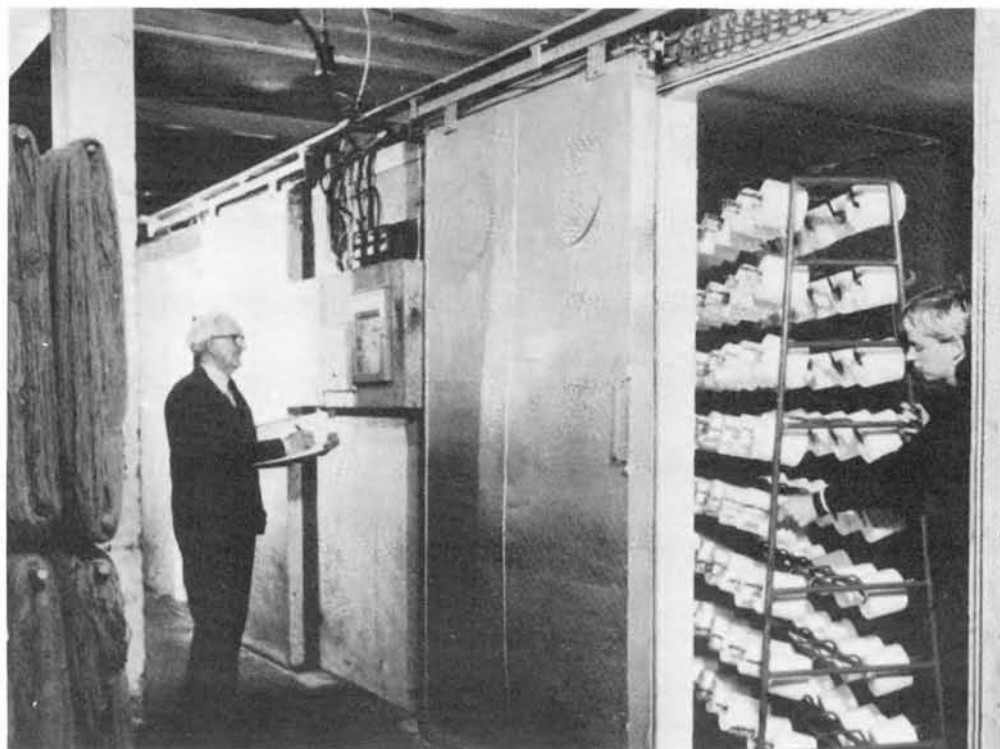
Figure 3 The dehumidification chamber at Kangol Wear Ltd. The Electricity Council
