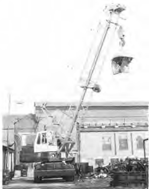
Figure 13 A mechanical mobile crane handles scrap with a magnet. Jones Cranes Ltd.
