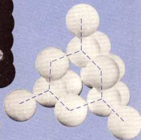
d. Tetrahedral packing – built up in such a way that each sphere forms the centre of a regular tetrahedron, whilst the four spheres surrounding it have their centres at the four corners of the tetrahedron. This again is a more open kind of packing.
