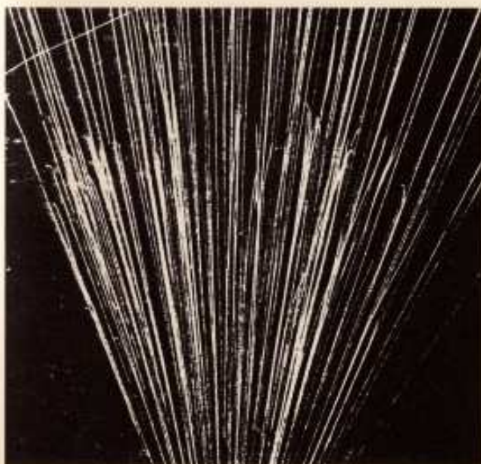
Disintegration of a nitrogen nucleus by an alpha particle. A.E.R.E. Harwell
