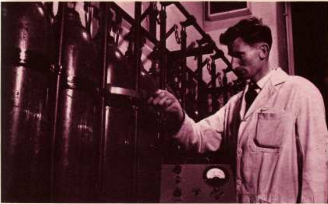
Using a level gauge to find the level of CO 2 in cylinders. U.K. Atomic Energy Authority
