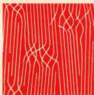
e. Stretching of crystalline polymers results in further alignment of the molecular chains and increased strength. Nylon and Terylene filaments are stretched to convert them into textile fibres.
