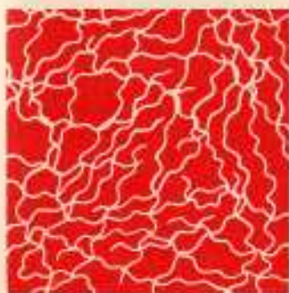
a. Random arrangement of molecular chains of different lengths with the chains continuously coiling and uncoiling. The intermolecular forces are weak and the polymers, which are soft and flexible, are classified as rubbers.
