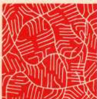
f. In some polymers, the molecular chains are branched and the branches may crystallize among themselves.
