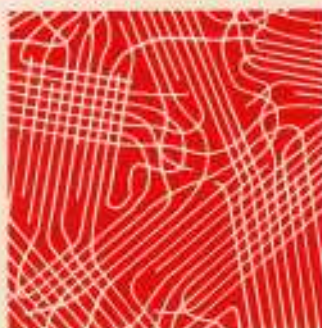
d. Several chains lie parallel to one another for all or part of their length to produce a close-packed orderly arrangement - as occurs in a number of thermoplastics. These regions of order are described as being crystalline, and the intermolecular forces between the chains are much stronger.
