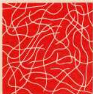
b. Forces between the chains are stronger and the chains less flexible to give an amorphous structure typical of many thermoplastics.
