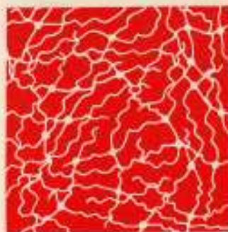
c. Cross-linking between the chains creates, in effect, a single giant molecule - as in thermosetting plastics such as Bakelite.
