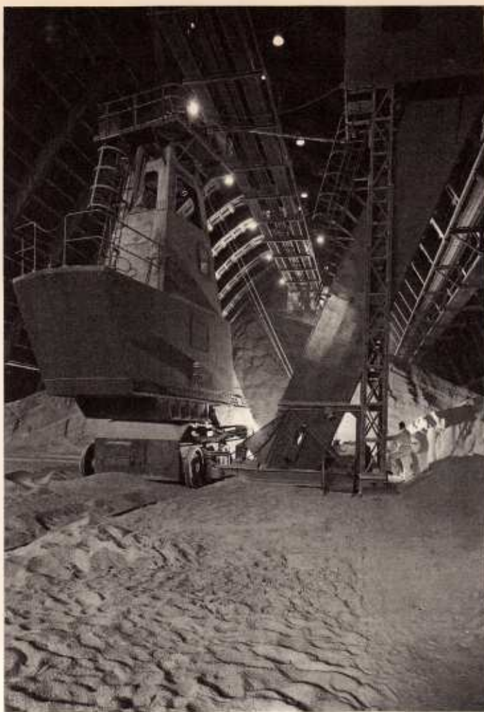
Large-scale storage of nitrogenous fertilizer made from petroleum. The 'harvester' machine transfers several hundred tons of fertilizer daily to an overhead conveyor which carries it to a bagging plant.
