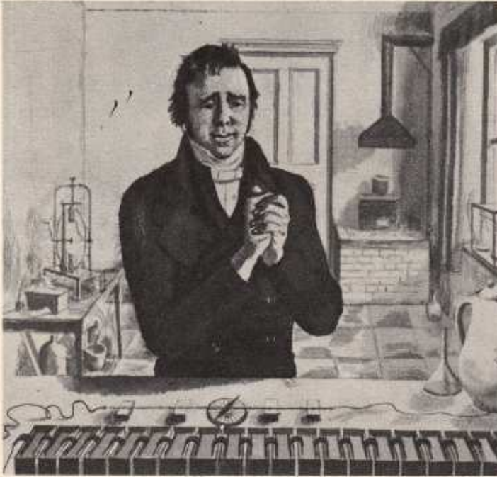
The Danish scientist Oersted discovers the magnetic effect of an electric current. He found that a magnetic needle placed parallel to a current-carrying wire was deflected. From 'An Illustrated History of Science' by F. Sherwood Taylor
