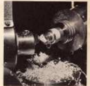
Turning a corneal contact lens with a diamond tool. Made of acrylic resin, the finished lens is only about 8 mm in diameter and 0.1 mm thick. Natural diamond is used here. De Beers.
