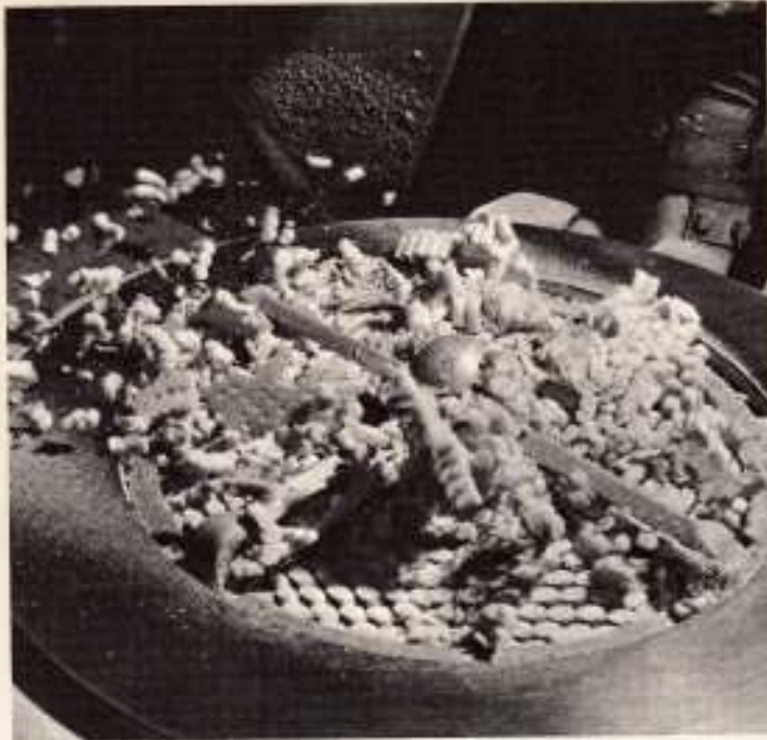
Modern soap manufacture is a continuous process. Here toilet soap is passing out of the second refiner. Colour and scent are then added, and the soap is refined twice more. Unilever
