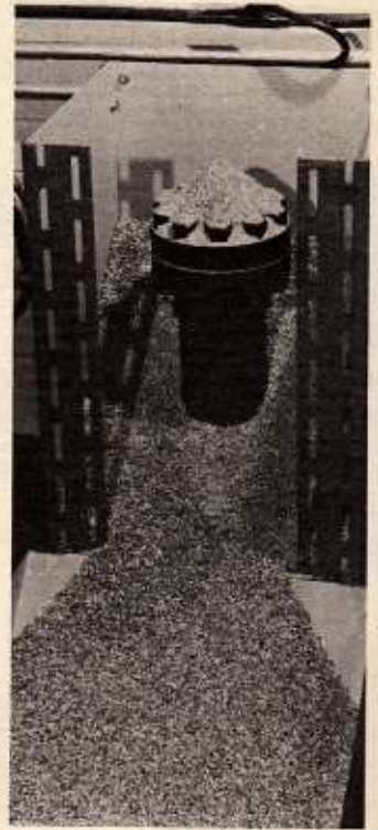
Autoclave for making quartz. The insulating material is packed in the box round the furnace as lagging to prevent heat loss.
