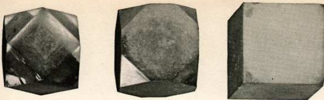
Alum crystals showing octahedral (left), and cubic (right) forms and combinations of the two.
