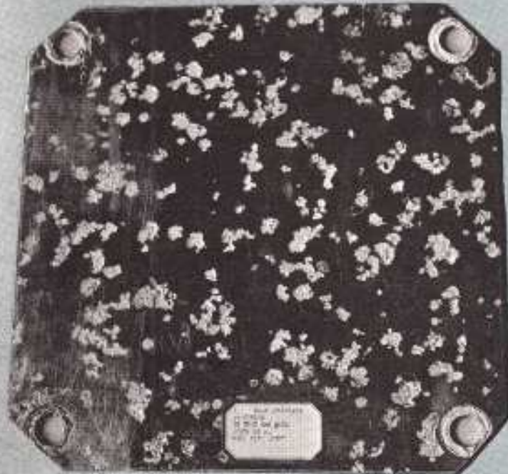
Pitting in a metal surface resulting from local corrosion under marine organisms that have become attached to the plate during immersion in sea-water.
