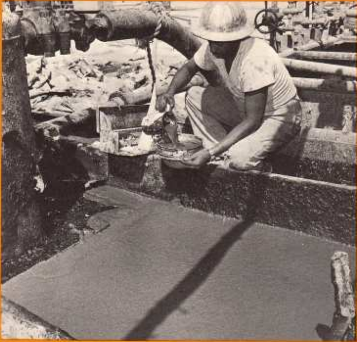
Drilling mud used as a lubricant in drilling for oil. Shell.
