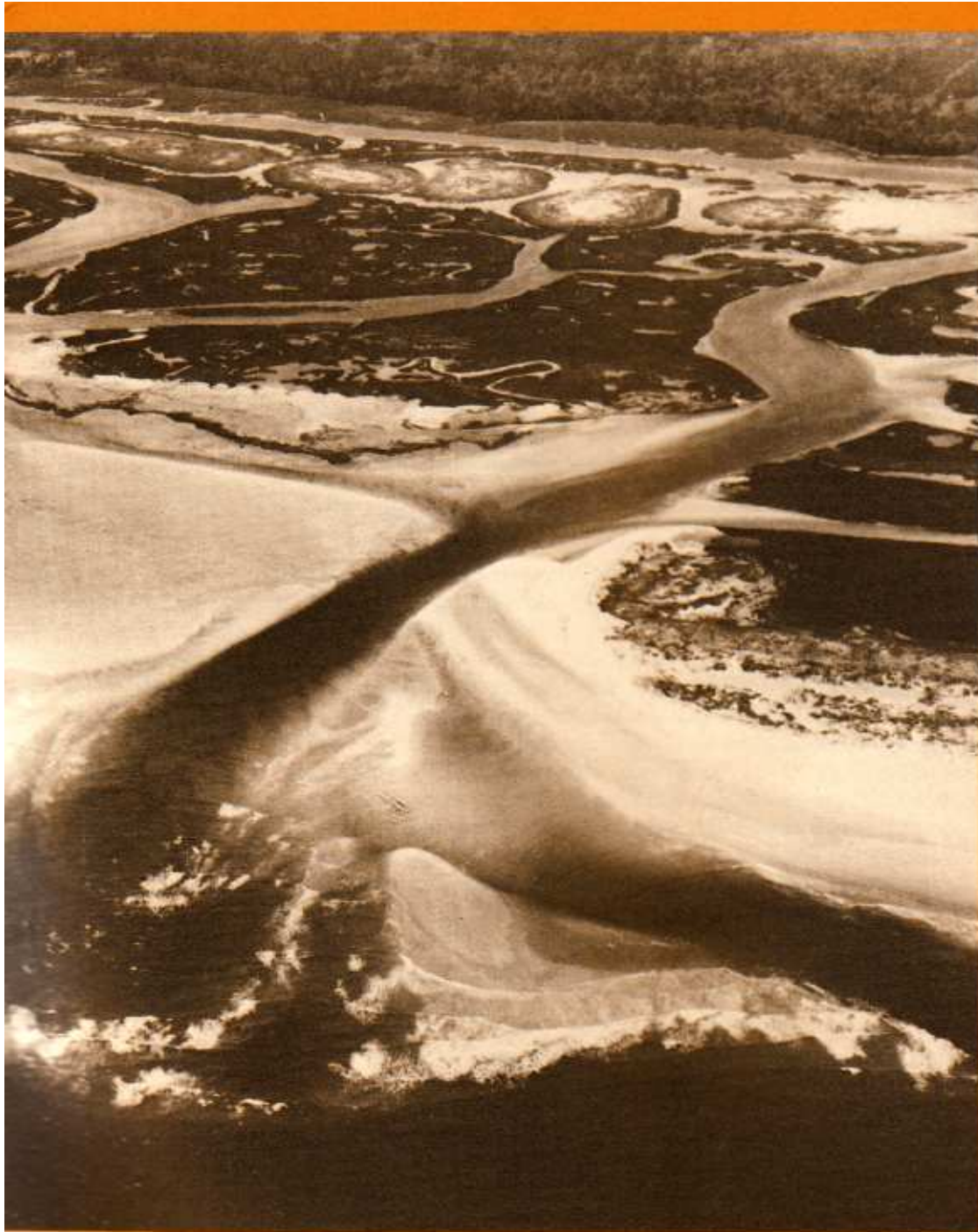
Mud carried in colloidal suspension in rivers settles when it meets the salt water of the sea at the river mouth. Aerofilms Ltd.
