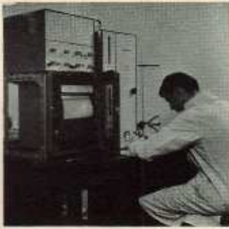
Standard equipment in most industrial chemical laboratories is gas chromatography apparatus for making quick and accurate analyses of substances. British Hydrocarbon Chemicals.
