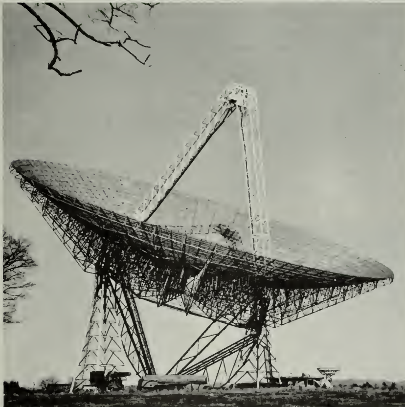
Left: the parabolic surface of a radio telescope reflects radio waves from space to a detector supported at the focus.
