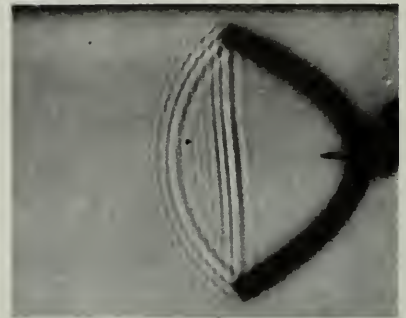
Above: A ripple tank shadow showing how circular waves produced at the focus of a parabolic wall are reflected from the wall into straight waves.
