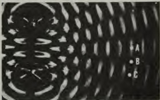
Fig. 1 An interference pattern in water. Two point sources vibrating in phase generate waves in a ripple tank. A and C are points of maximum disturbance (in opposite directions) and B is a point of minimum disturbance.
