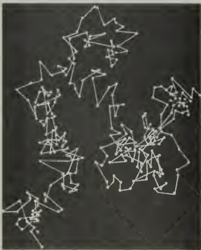
Record of a particle in Brownian motion. Successive positions, recorded every 20 seconds, are connected by straight lines. The actual paths between recorded positions would be as erratic as the overall path.
