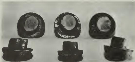
Fig. 1 Broken coupling pins from colliding freight cars.
