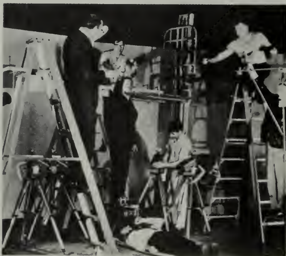
Fig. 4 Catching the seven scattered balls to avoid tangling in the wires from which they hang. The photographer and the camera are on the floor. The four stroboscopes are seen on tripods in the lower center of the picture.
