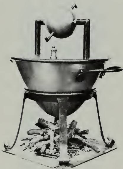
A model of Heron's aeolipile. Steam produced in the boiler escapes through the nozzles on the sphere, causing it to rotate.
