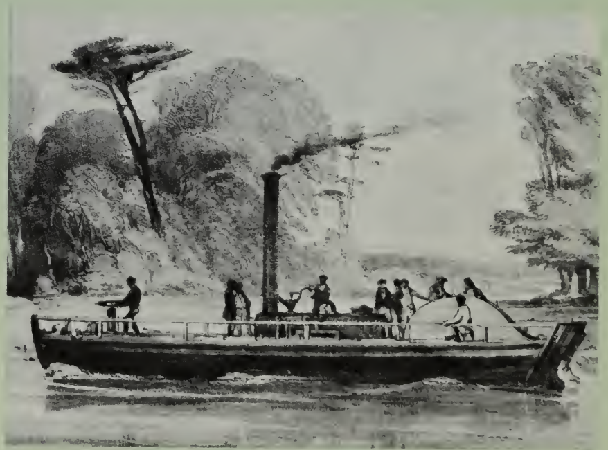
The "Charlotte Dundas," the first practical steamboat, built by William Symington, an engineer who had patented his own improved steam engine. It was tried out on the Forth and Clyde Canal in 1801.
