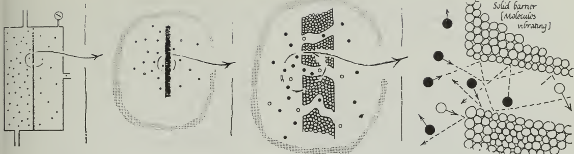
FIG. 25-15. SEPARATION OF URANIUM ISOTOPES BY DIFFUSION OF UF_6 THROUGH A POROUS BARRIER Gas molecules hit the barrier, and the walls of its pores, many times—net result: a few get through.
