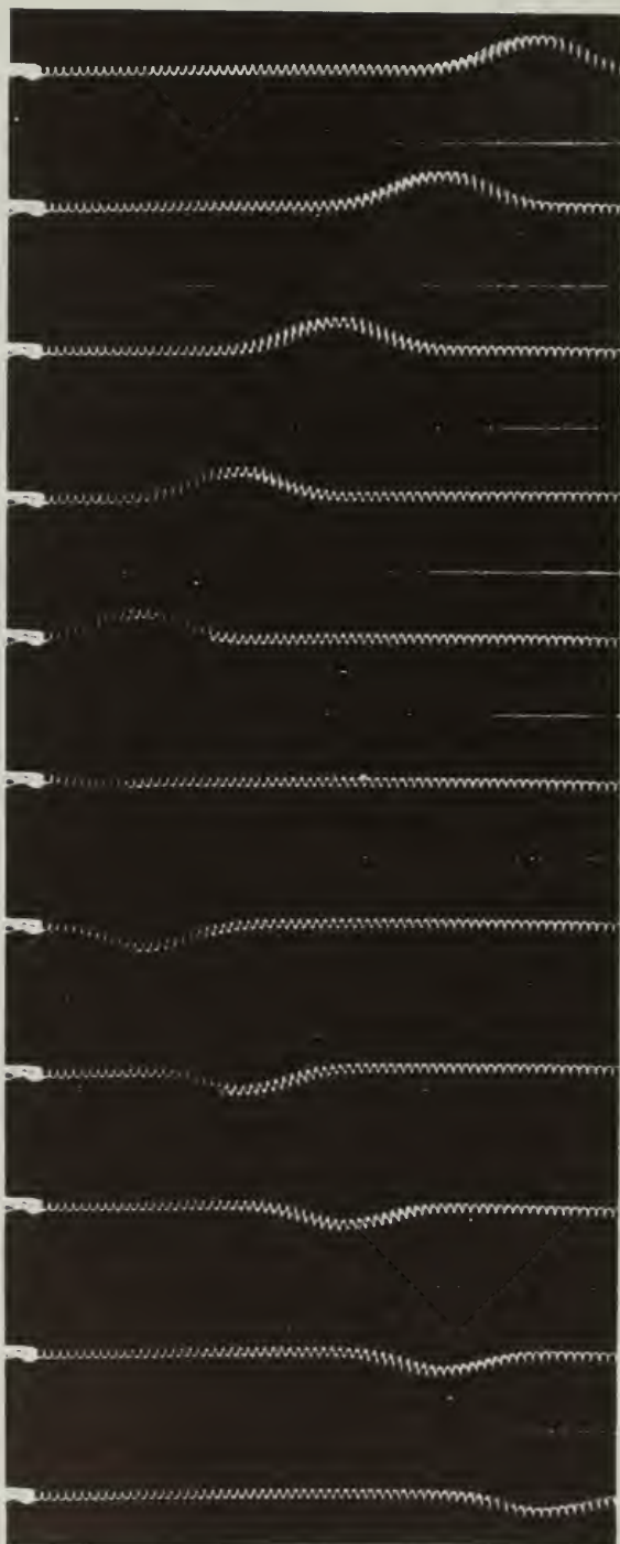
FIGURE 17.1 This sequence of photographs shows a pulse traveling to the left on a long coil spring. The pulse is reflected by the fixed end of the spring and the reflected pulse is inverted. (From Physical Science Study Committee: Physics. Boston, D. C. Heath & Co., 1960. Copyright, Educational Services Inc.)
