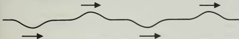
FIGURE 17.5 We can send a succession of pulses along a long rope by jerking one end up and down.
