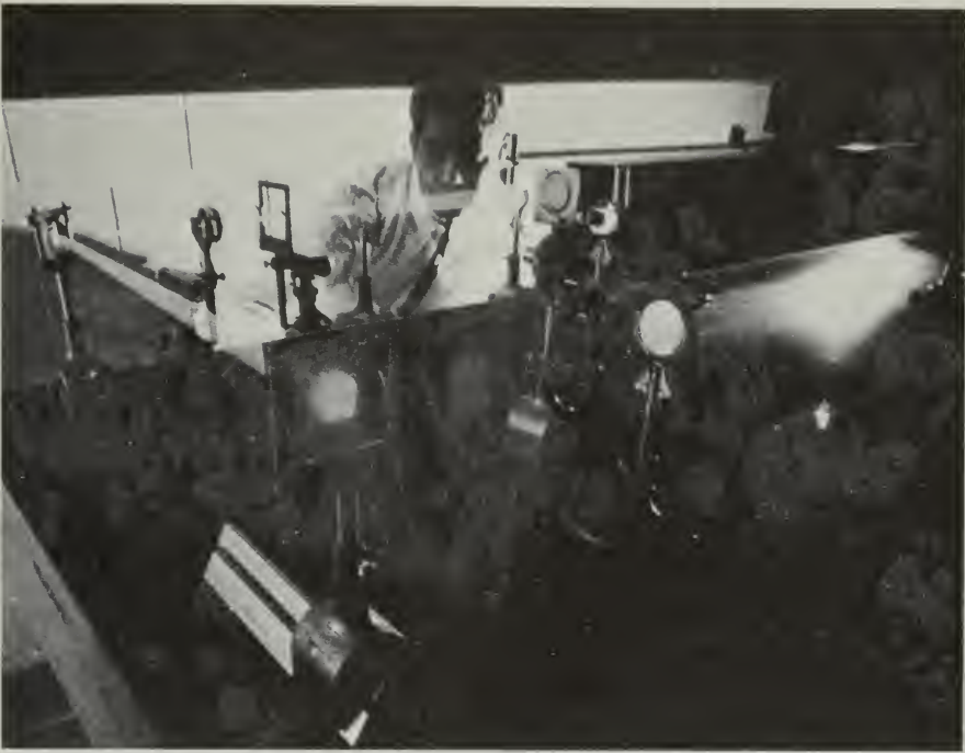
ACOUSTICAL HOLOGRAPHY. Acoustical wavefronts reflected from irregular surfaces can be recorded and reconstructed with coherent laser light. An advantage over conventional holography is that optically opaque gases and liquids can be penetrated. The experiment shown is in progress at the McDonnell Douglas Corp. —FIG. 6
