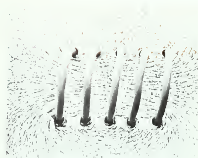
Iron filings in the magnetic field produced by current in a coil of wire.
