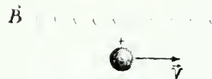
(a) When the charge q moves with velocity \vec{v} perpendicular to \vec{B} ,
