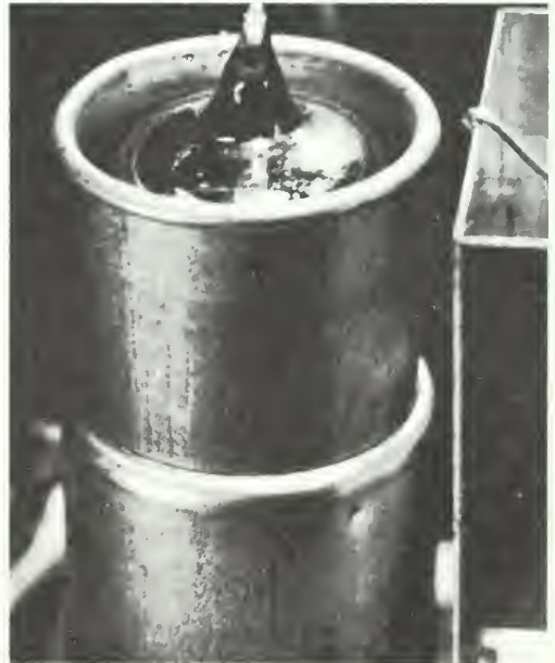
Closeup of a tube in the tuning section of the TV set on the left. Surrounding the tube is a collapsible metal shield. Partly shielded tubes can be seen elsewhere in that photo.
