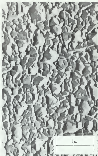
The surface of a mirror as shown by a scanning electron microscope. The surface is a 3-micron thick aluminum film. The magnification here is nearly 26,000 times. ( \mu stands for micron; 1\mu = 10^{-6} \text{ m} .)
