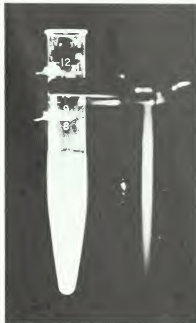
Starting about 6 years after Fermi's speculation of 1934, it was found possible, by a variety of methods, to create transuranium elements. The new elements up to Z = 106 are listed below. A tiny sample of one of them, curium-244, dissolved in a test tube of water, is shown in the 5-min exposure above (by light produced when the radiation interacts with the surrounding matter).
