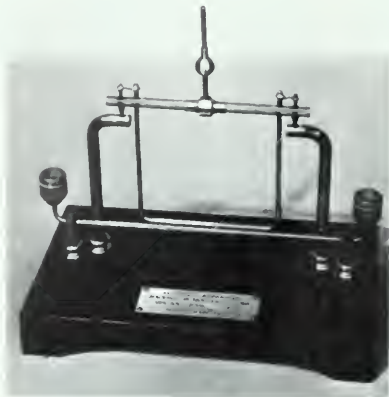
Replica of Ampère's current balance. The essential part is a fixed horizontal wire (foreground), and just behind it, hanging from a hinged support, a shorter segment of wire. Current is produced in both wires, and the force between them is measured.
