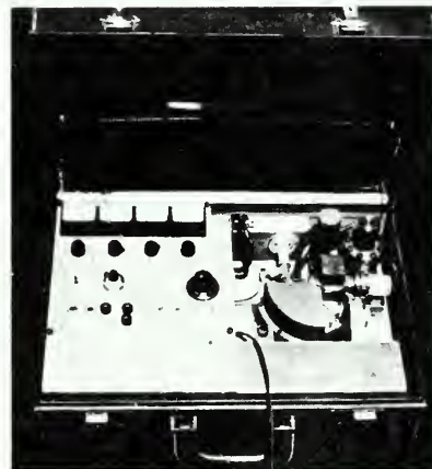
Some mass spectrometers are portable; small ones similar to this are carried aloft by rocket or balloon for the analysis of the gases in the upper atmosphere.
