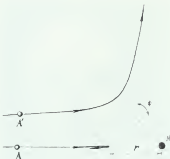
Paths of two \alpha particles A and A' approaching a nucleus N. (Based on Rutherford, Philosophical Magazine , Vol. 21, 1911, p. 669.)
