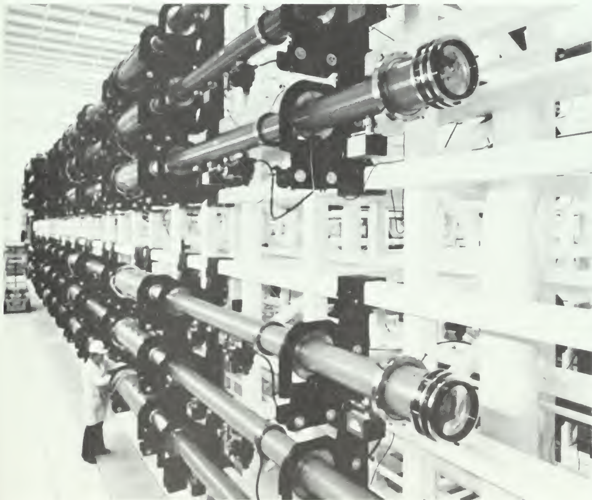
These powerful lasers are part of the experimental Shiva fusion device. The energy supplied by the lasers is directed onto a tiny fuel pellet, causing the pellet to implode and thus release energy.
