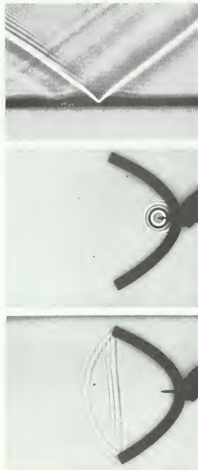
Above: A ripple tank shadow showing how circular waves produced at the focus of a parabolic wall are reflected from the wall into straight waves.
