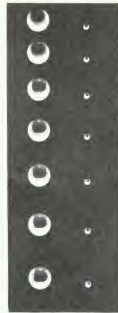
A stroboscopic photograph of two freely falling balls of unequal weight. The picture shows the last part of the total path. The balls had been released simultaneously. The time interval between images is 0.03 sec.
