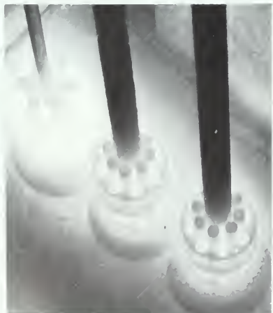
The glow in the photograph is caused when gamma rays emitted by radioactive cobalt cylinders interact with the surrounding pool of water.
