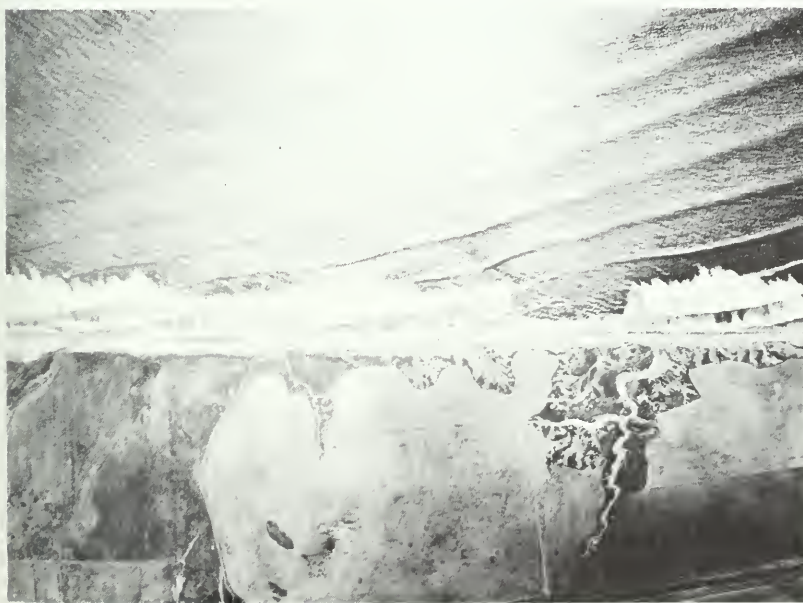
Top: Ripples on water (coming from the left) encounter the shallow region over the corner of a submerged glass plate. Bottom: Ripples on water (coming from the left) encounter a shallow region over a glass plate placed at an angle to the wave fronts.
