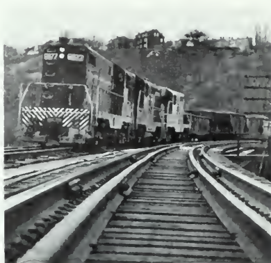
An engine starting abruptly can start a displacement wave along a line of cars.
