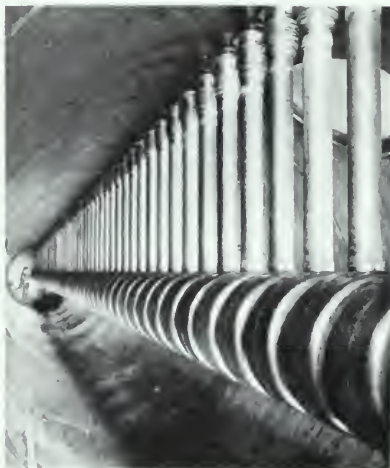
An inside view of the heavy ion linear accelerator at Berkeley, California. In this device electric fields accelerate charged atoms to high energies.
