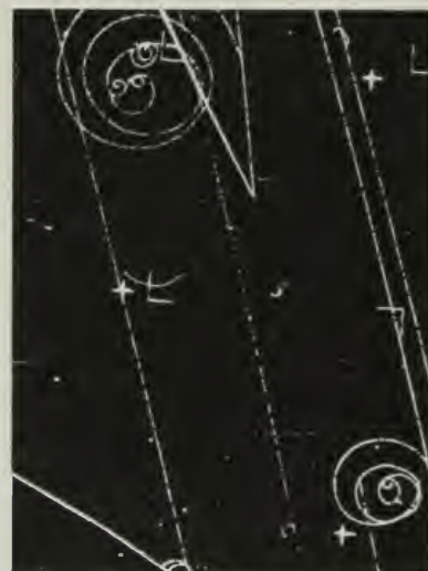
In this bubble chamber picture, a neutron is produced at the bottom, at the end of the \frac{1}{2} " long track, near the + mark. This neutron in turn causes a reaction near the center of the plate. (Neutral particles do not leave tracks in bubble chambers.)
