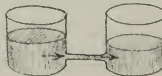
Fig. 21-9 An analogy: The rate of flow of water depends upon the difference in height of the water in the two tanks and upon the resistance the pipe offers to the flow of water.
