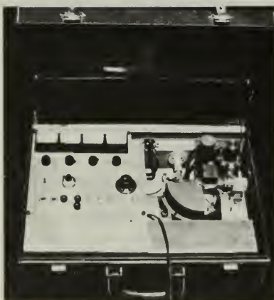
Some mass spectrometers are portable; small ones similar to this are carried aloft for analysis of the upper atmosphere.
