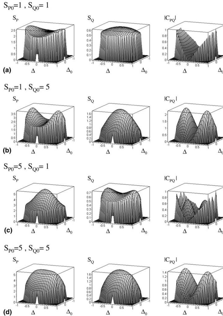
Fig. 2. Normalized noise of the field correlations in an OPO, as a function of the cavity detuning, for different pump noise conditions.  $S_p$ : noise of the sum of the amplitude quadratures  $p_+$ ,  $S_q$ : noise of the sum of the phase-related quadratures  $q_+$ ,  $|C_{pq}|$ : absolute value of correlations between the sum of amplitude and phase-related fluctuations. Parameters are  $\gamma = 0.01$ ,  $\gamma_0 = 0.05$ ,  $\Omega = 2\gamma/\tau$ ,  $\sigma = 2$ .
