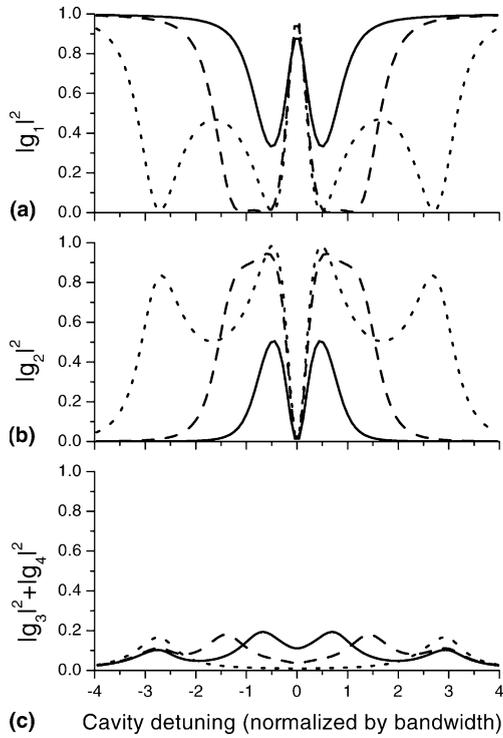
Fig. 4. These curves show the behaviour of the coefficients appearing in Eq. (21) as a function of cavity detuning (in units of cavity bandwidth). A finesse  $F = 270$  is assumed. Continuous line:  $\Omega = \delta\omega/\sqrt{2}$ ; dashed line:  $\Omega = \sqrt{2} \delta\omega$ ; dotted line:  $\Omega = 2\sqrt{2} \delta\omega$ . (a)  $|g_1(\Omega)|^2$ , (b)  $|g_2(\Omega)|^2$ , (c)  $|g_3(\Omega)|^2 + |g_4(\Omega)|^2$ .
