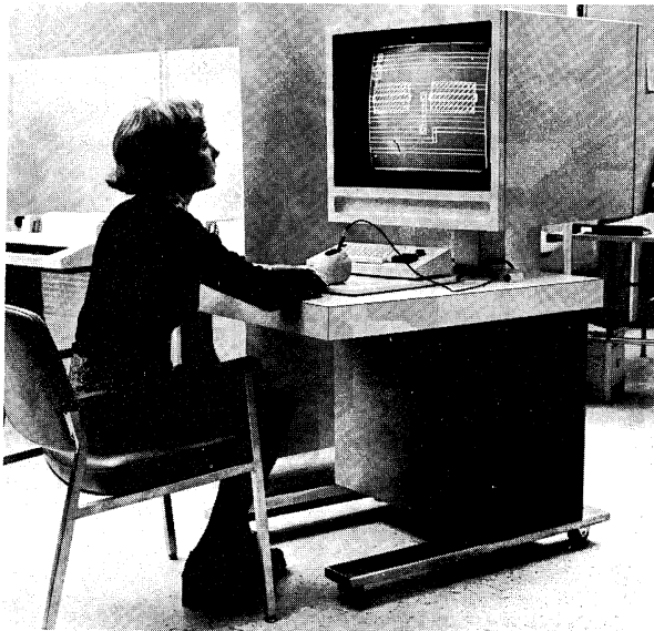
Sections of the integrated circuit, much enlarged, can be checked on a visual display unit.
