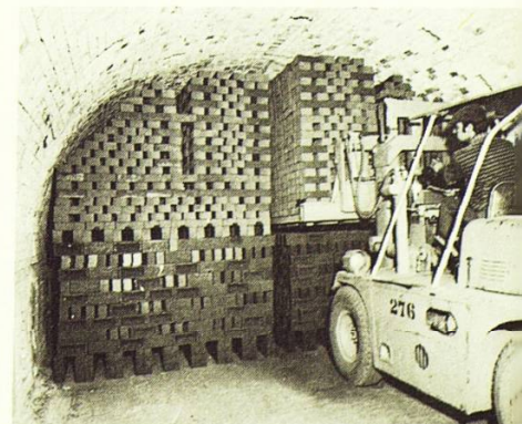
Left: Clay scooped out with a drag line and bucket Centre: Brick presses, each cutting two bricks at a time Right: A large brick kiln being filled with bricks
