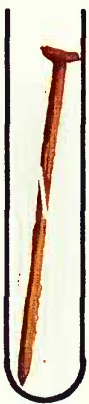
6 Copper plated nail (scratched) – you can copper-plate by placing in copper sulphate solution.
