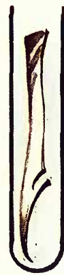
2 Scratched piece of tinplate. Also try scratching tin cans and leaving in various places.
