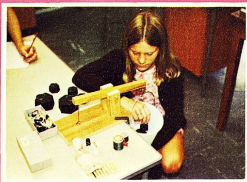
Thread breaker in use with load
