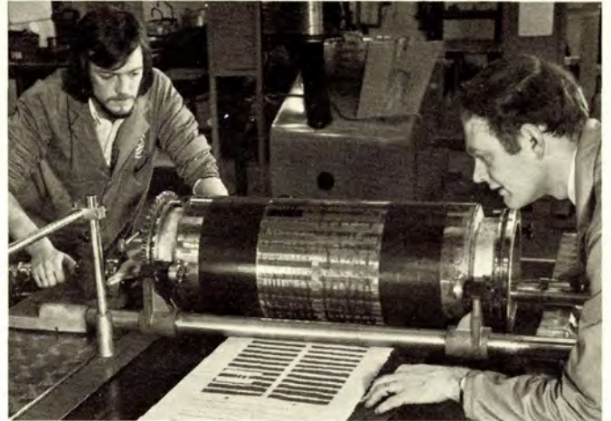
Here a dye is being tested. The dye is rolled out on to the fabric to make a pattern. This is called printing .
