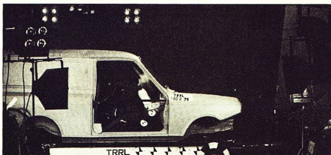
A car travelling at 30 mph at moment of impact. Driver with seat belt on.
