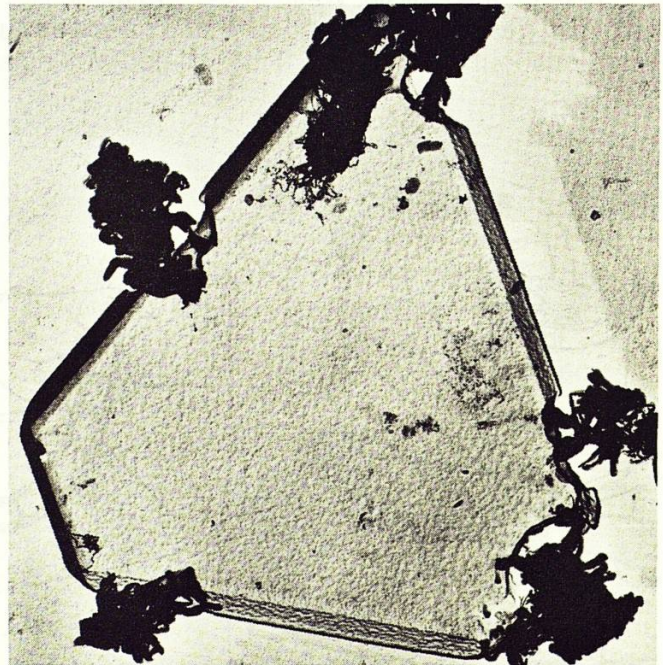
The emulsion is made up of very small crystals of silver halide. This crystal is being developed — it is beginning to turn black. (Magnification 12 000 times.)
