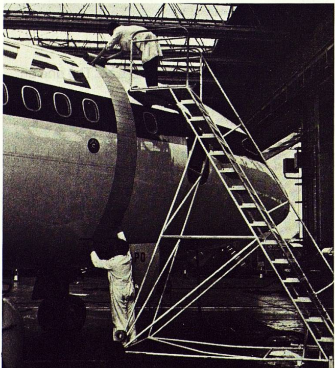
More powerful X-rays are used in industry. Here a BEA Trident is being inspected by radiography.
