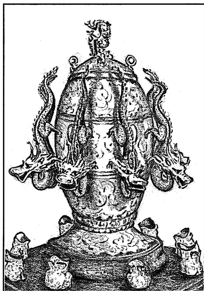
Figure 7 A Chinese earthquake detector invented in 132 AD
