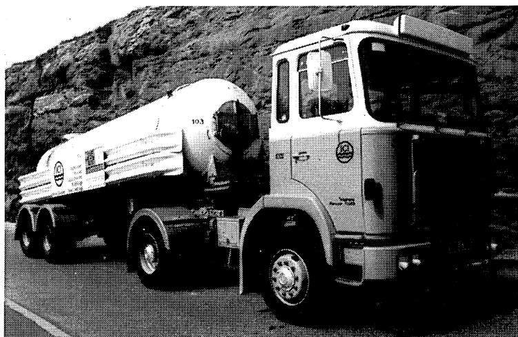
Figure 3 A road tanker carrying chlorine
